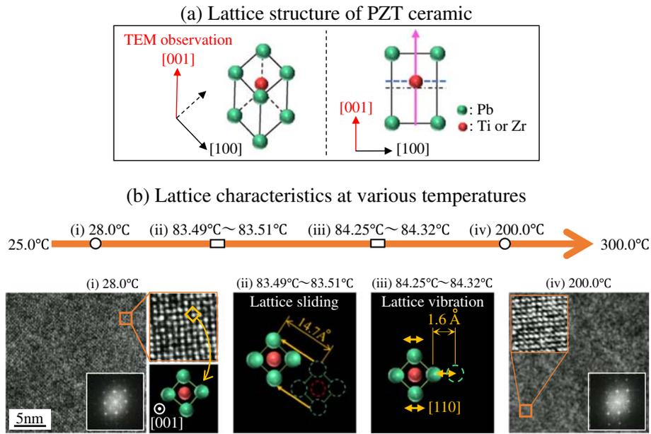
Fig. 1. (a) Lattice structure of the PZT ceramic and (b) lattice characteristics at various temperatures.
