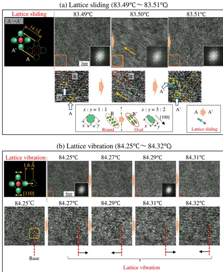
Fig. 2. Lattice motion of the tetragonal structure during heating: (a) sliding and (b) vibration.
