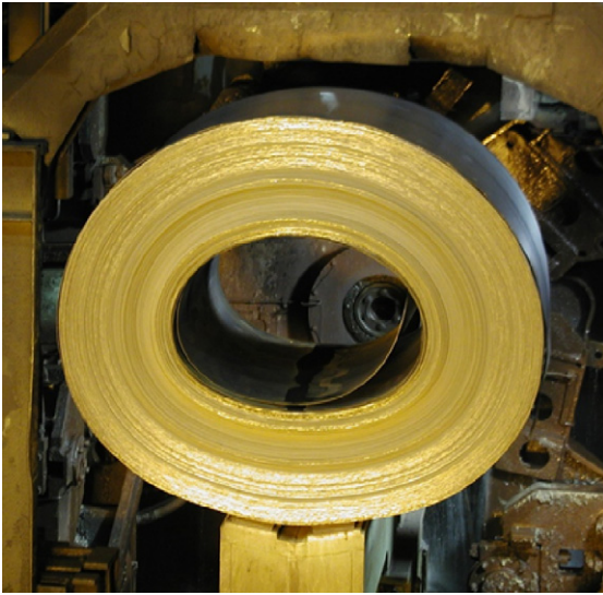
Fig. 1. An example of asymmetric contraction of hot coil after coiling.
