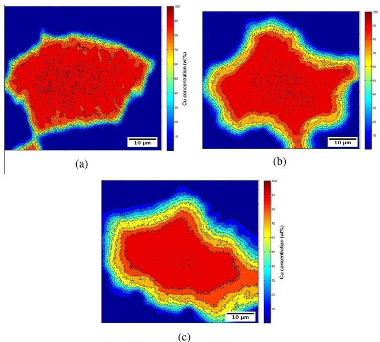
Figure 1. Copper concentration by area for compacts sintered for 30 min at (a) 700 °C, (b) 800 °C and (c) 900 °C.
