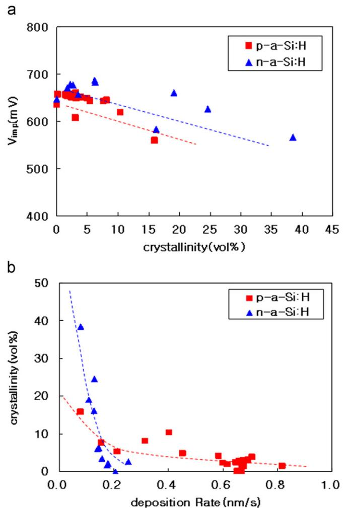
Fig. 2. (a) The relationship between the implied open circuit voltage and crystalline volume fraction in each a-Si:H thin film. (b) The relationship between the deposition rate and crystalline volume fraction in each a-Si:H thin film.
