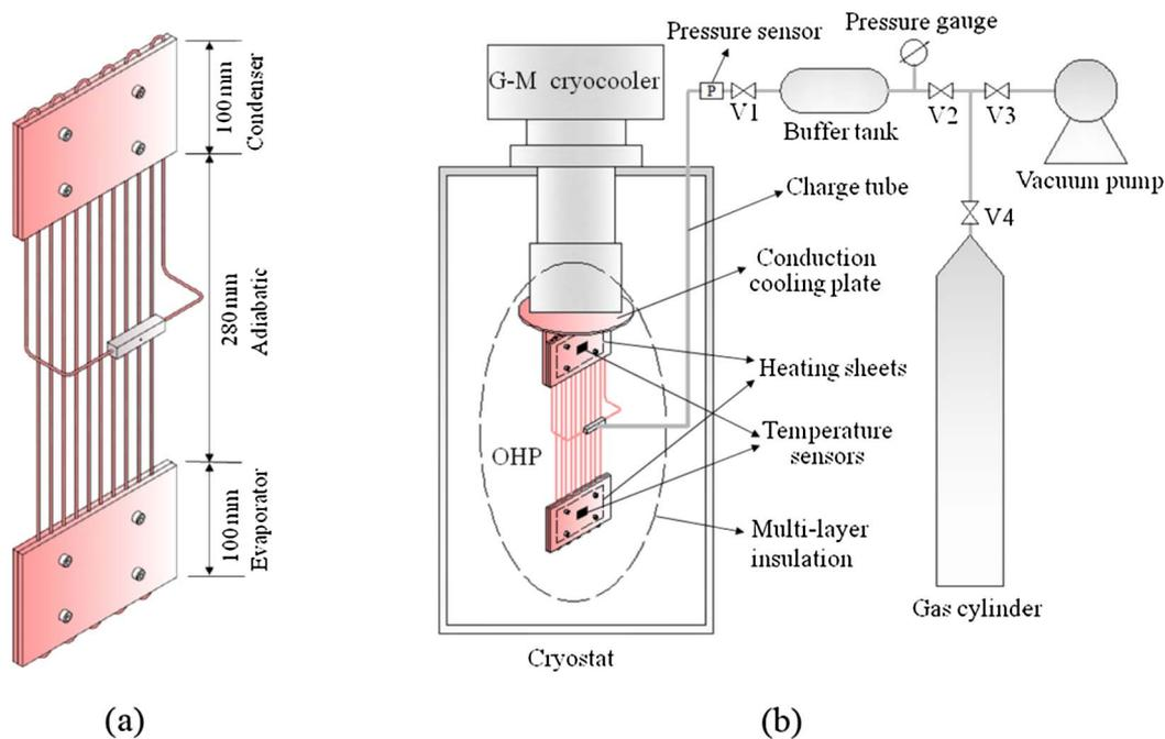
Fig. 1. (a) The configuration of the cryogenic OHP and (b) schematic illustration of the experimental apparatus.
