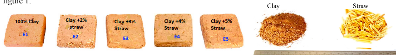
Figure 1: View of composite samples with different percentages of straw
