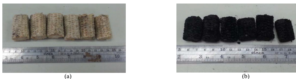
Fig. 1. Feedstock (a) raw empty cobs; (b) torrefied empty cobs
