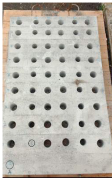
Fig. 1. Specimen position in the experimental concrete wall
