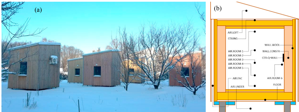
Fig. 1. Testing buildings: (a) site overview; (b) cross-section of the building with main temperature and air humidity sensor location.
