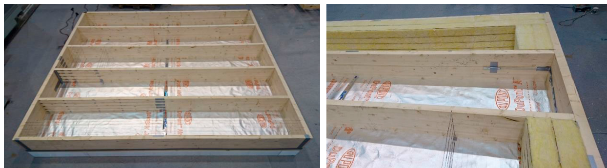
Fig. 1. Photo showing the timber frame test section under construction with a reflective foil at the hot side of the cavities and thermocouples mounted for measuring temperatures inside the cavities. Edge insulation partly mounted, (right).
