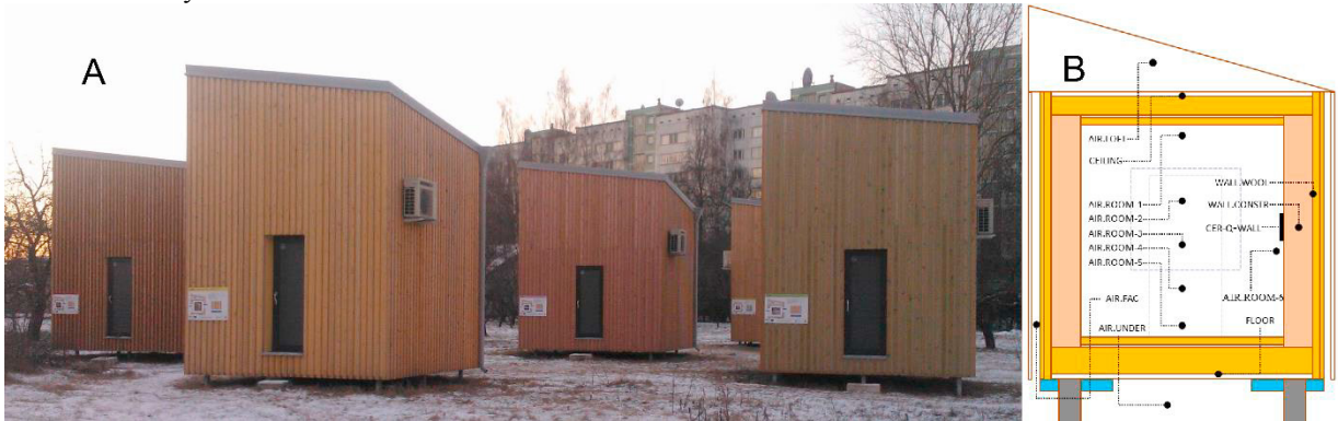
Fig. 1. (a) Test ground (b) Schematic sensor positions.
