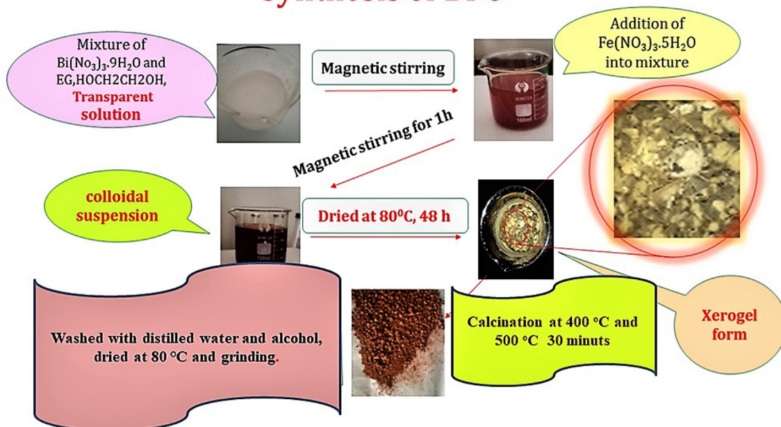
Fig. 1. Method employed for producing BFO nanoparticles via the sol-gel method.
