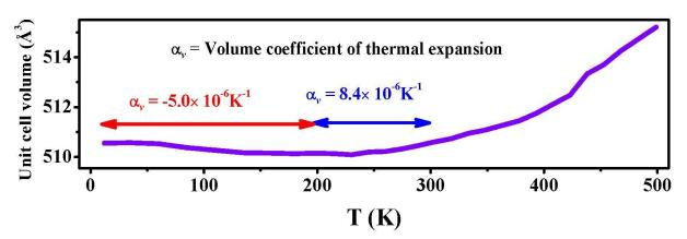
Ferrimagnetic  $Ho_2Fe_{16.5}Cr_{0.5}$  having  $T_C = 394$  K, shows negligible thermal expansion below 300 K due to magnetovolume effect.
