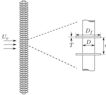
**Fig. 1.** Isolated finned cylinder geometry consisting of a base cylinder of diameter  $D$  with circular fins having thickness  $T$  and diameter  $D_f$ , separated by pitch  $c$ .
