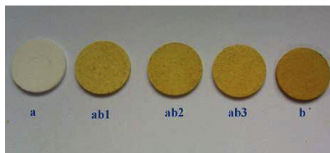
Fig. 2. Disc samples for electrical properties measurements. (a) Acetaminophen (100%); (ab1) Acetaminophen (75%)/Curcumin (25%); (ab2) Acetaminophen (50%)/Curcumin (50%); (ab3) Acetaminophen (25%)/Curcumin (75%); (b) Curcumin (100%).
