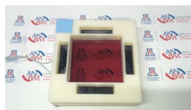
Fig. 1. Left: Typical polymer EC device architecture for glass/ITO substrate. From top to bottom, the 7 layers are glass/ITO/ECP/electrolyte/charge storage/ITO/glass where ITO serves as the transparent electrode and glass is the substrate material; Right: a magenta color EC device consist of the 7-layer structure, which was fabricated at the Center for Applied Nanobioscience and Medicine. The magenta EC polymer was provided by Dr. J.R. Reynolds' group at Georgia tech, and the device was assembled according to Ref. [10].
