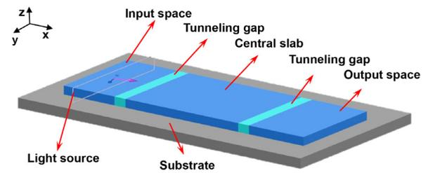
Fig. 2. Optical structures of the ROTE in the FDTD simulation.
