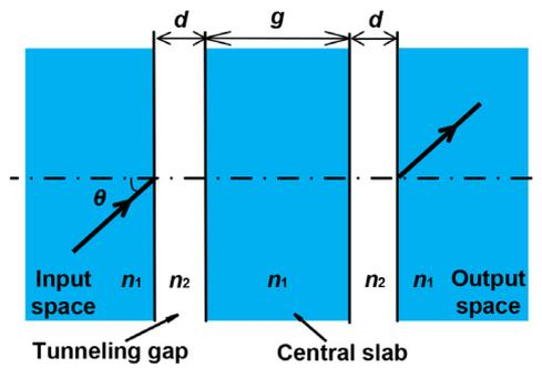
Fig. 1. Schematic diagram of the ROTE structure.
