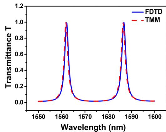
Fig. 3. Transmission spectra of ROTE obtained by the TMM and the FDTD when the light is in P-polarization.
