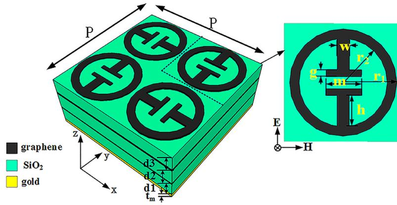
Fig. 1. Schematic of the proposed absorber. The geometrical parameters of the proposed structure are:  $P = 5 \mu\text{m}$ ,  $w = 0.3 \mu\text{m}$ ,  $g = 0.15 \mu\text{m}$ ,  $m = 0.8 \mu\text{m}$ ,  $h = 0.4 \mu\text{m}$ .
