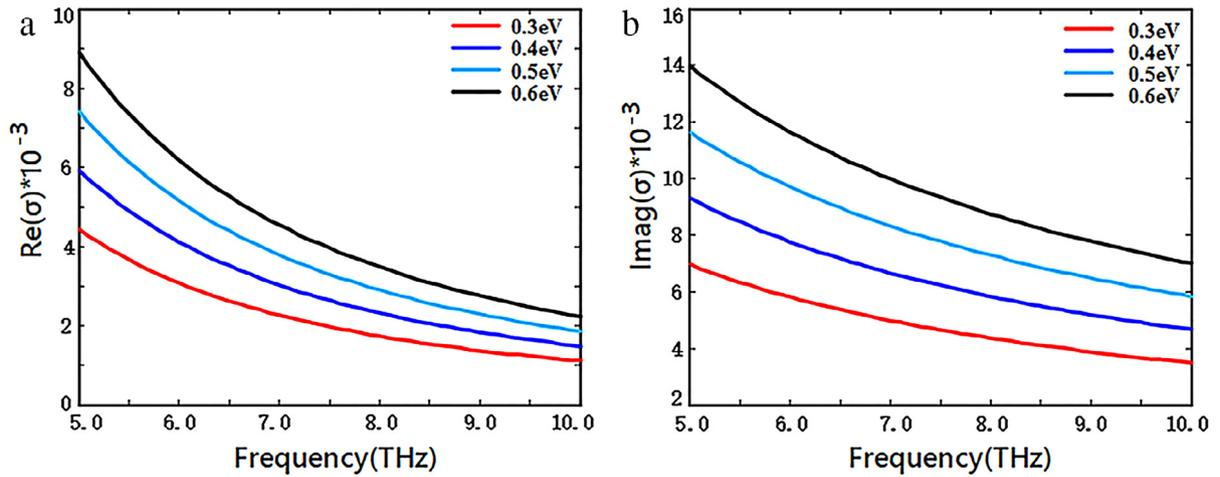
Fig. 2. Graphene conductivity (a) real part (b) imagine part at different Fermi level.
