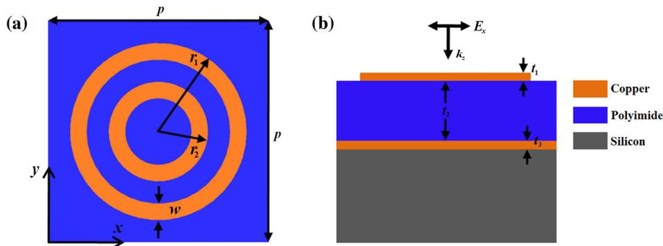
Fig. 1. (a) Schematic of the circular ring resonators of the proposed PMA and (b) cross section of the complete PMA.
