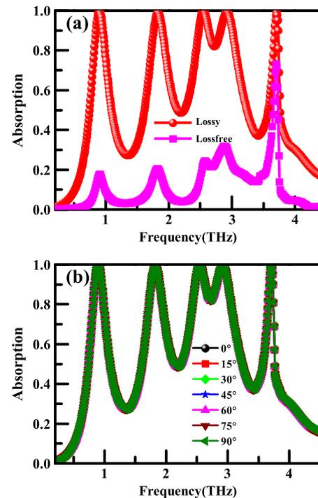
Fig. 2. (a) Calculated absorption spectra of the proposed five-band PMA with two different loss properties (lossy and lossfree) of dielectric, respectively. (b) Calculated absorption spectra with different polarization angles of incident terahertz wave.
