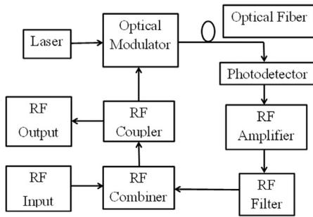
Fig. 1. Schematic diagram of a single-loop OEO.
