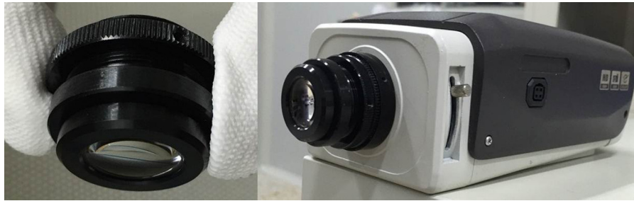
Fig. 1. Single-lens camera developed by authors. Effective focal length (EFL) is 35 mm, f/2.4 .
