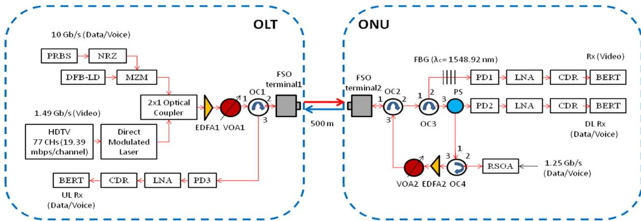
Fig. 1. Experimental setup for next-generation bidirectional Triple-play services using RSOA based WDM-RoFSO-PON.
