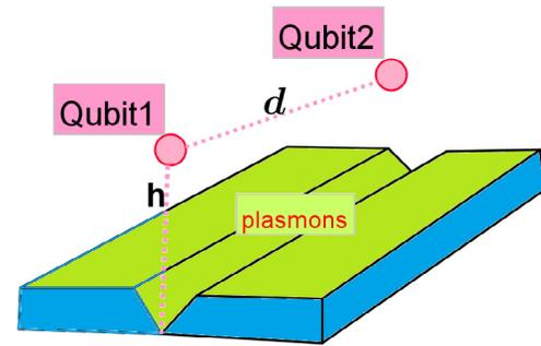
Fig. 1. The composite NVC–PW system consisting of two identical NVCs in diamond nanocrystals and a 1D plasmonic waveguide.
