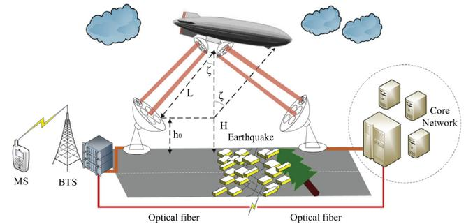
Fig. 1. The model of two-way relaying FSO communications for HAP-based broadband backhaul networks.
