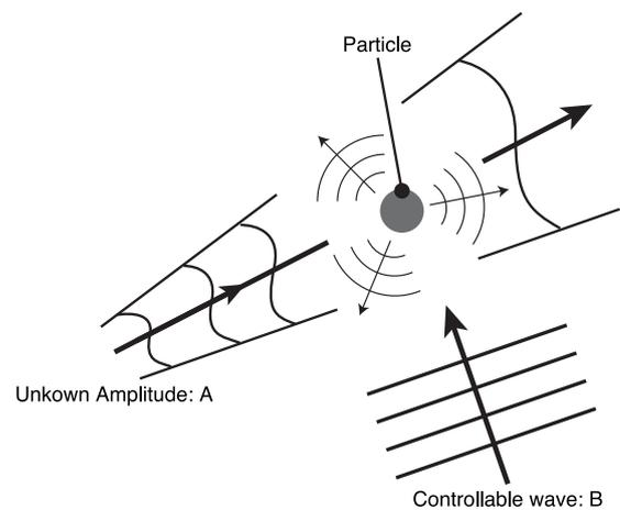
Fig. 2. Principle of non-perturbative field measurement with a highly scattering particle. The unknown electric field **A** wave is scattered by the particle. The polarization, amplitude, and phase of a second wave **B** are controlled to minimize the scattering.
