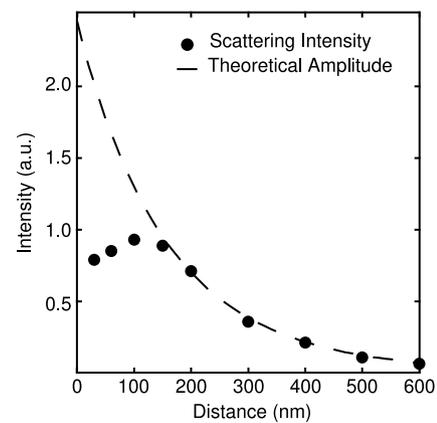
Fig. 1. Theoretical amplitude distribution and scattering intensity from a particle in the evanescent field. The amplitude distribution and scattering intensity depend on the distance between the surface and the particle.
