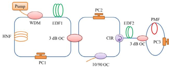
Fig. 1. Experimental setup of the multi-wavelength mode-locked fiber laser. EDF: erbium-doped fiber; WDM: wavelength division multiplexer; HNF: high nonlinearity fiber; PMF: polarization maintaining fiber; PC: polarization controller; OC: optical coupler; CIR: circulator.
