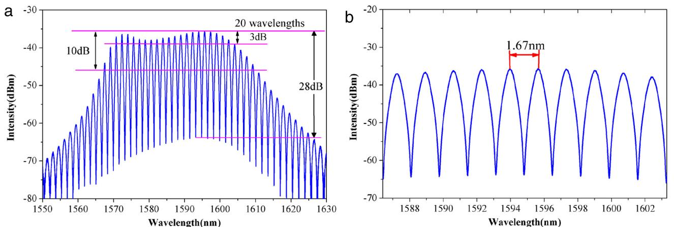
Fig. 3. (a) The output spectrum optimized by EDF2; (b) The enlarged output spectrum.
