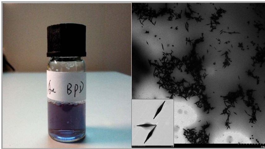
Fig. 1. Photograph of Au-NBPs solution and TEM image of the gold nanobipyramids.
