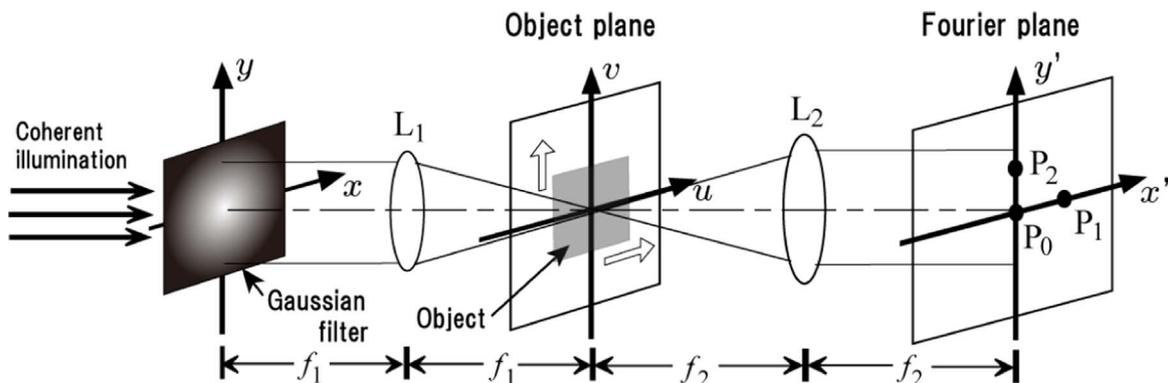
Fig. 1. Schematic diagram of the geometry of the scanning phase-retrieval system with a Gaussian-amplitude beam. The object function is reconstructed from intensities measured at three coordinates in the Fourier plane as a function of the object position.
