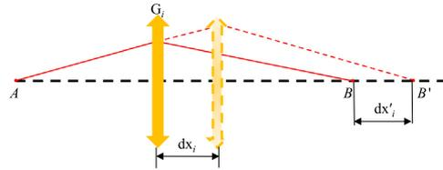
Fig.2. Notation of object and image in group moving for one single lens.
