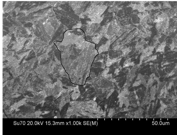
Fig. 1. SEM micrograph of the surface of P91, black outline represents a typical block.
