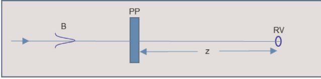
Fig. 1. Simple setup to generate the annular focusing of a beam.
