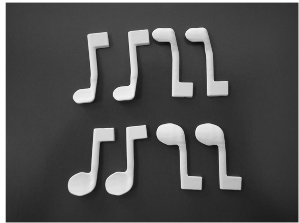
Fig. 1. The two types of ceramic cores for the turbine blade.
