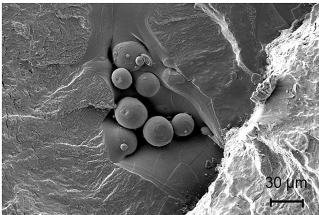
**Fig. 1.** Non-processed particles as nuclei for cracks: fracture surface of a sample with a colony of unmolten TiAl6V4 particles.
