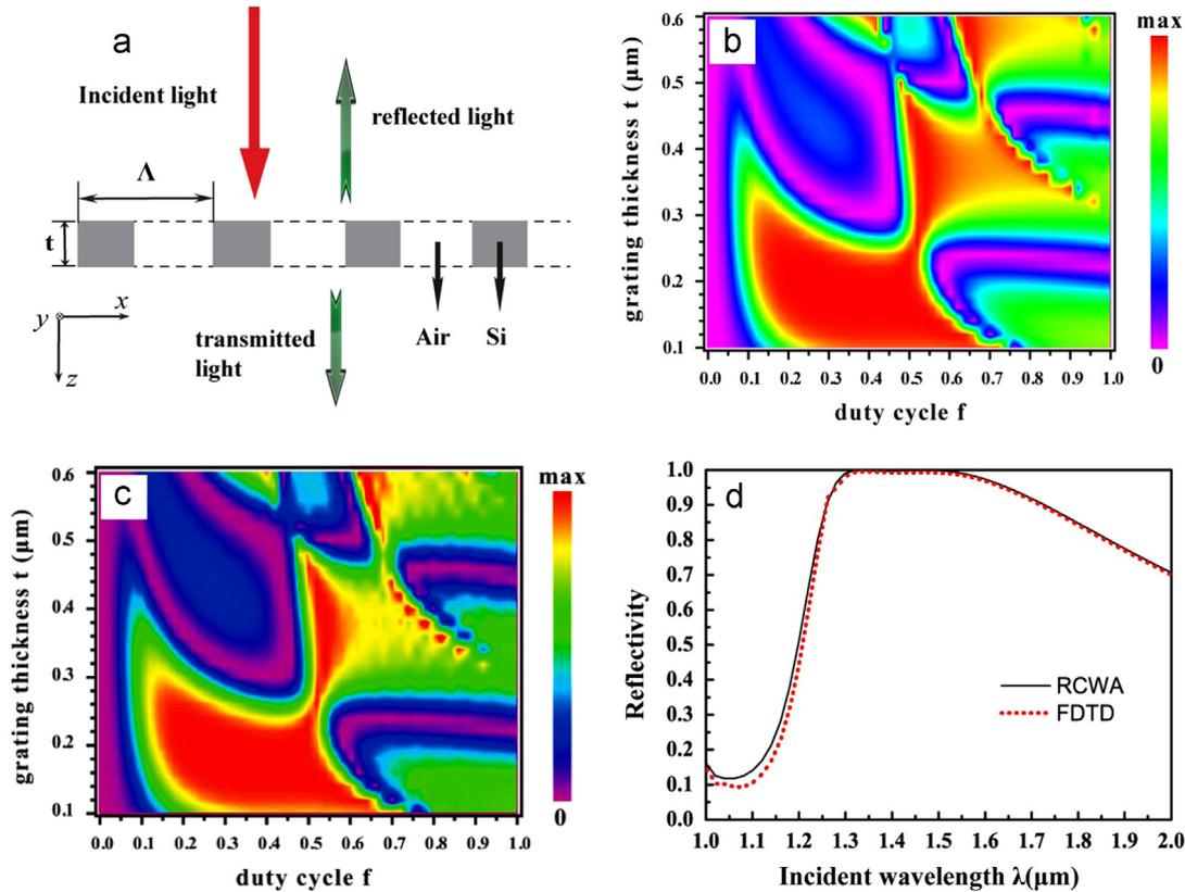
**Fig. 1.** (a) Schematic of a planar HCG structure. The reflectivity distributions calculated by (b) RCWA and (c) FDTD methods for the grating thickness  $t$  from  $0.1 \mu\text{m}$  to  $0.6 \mu\text{m}$  and the duty cycle  $f$  from 0 to 1. (d) Results from RCWA/FDTD methods when  $\Lambda = 1 \mu\text{m}$ ,  $t = 0.25 \mu\text{m}$  and  $f = 0.2$ . (For interpretation of the references to color in this figure, the reader is referred to the web version of this article.)
