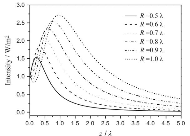
**Fig. 2.** The dependence of the whole intensity on  $z$  as  $x=y=0$  and  $I_0=1$  W/m<sup>2</sup> for different  $R$ .
