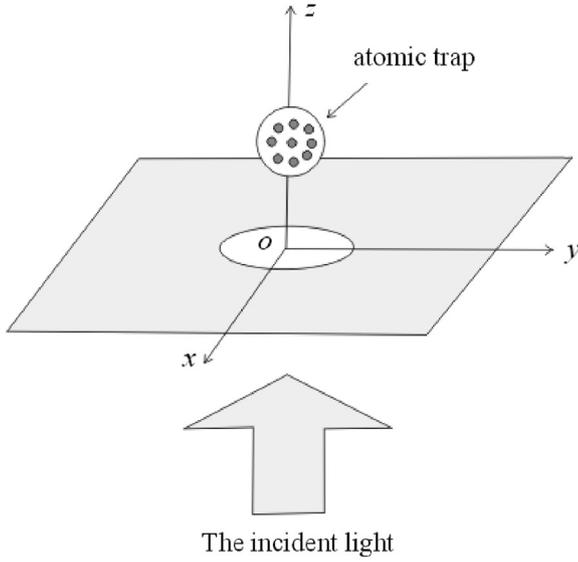
**Fig. 1.** Scheme diagram of the trapping of isolated cold atoms using the diffraction of a subwavelength thin circular aperture in the near field.
