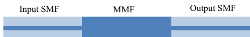
Fig. 1. Schematic diagram of the MMFI investigated in this work; (SMF, single mode fiber; MMF, multimode fiber).
