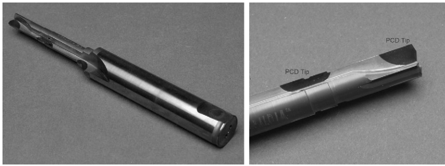
Fig. 1. Typical cutting tools with PCD tips on the cutting edges.
