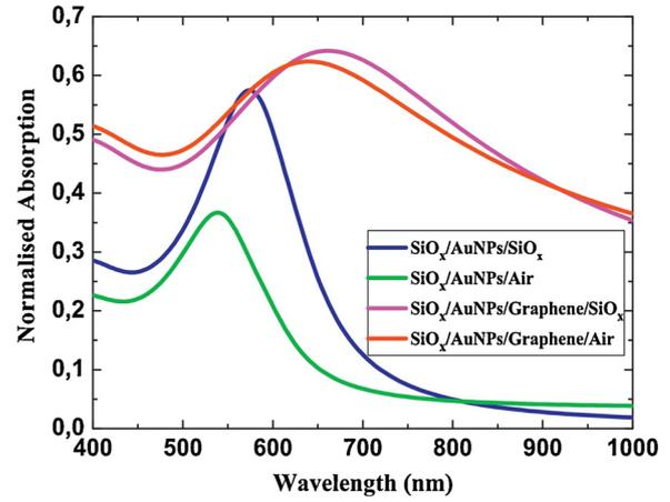
**Fig. 2.** Computed absorption spectra of AuNPs, in the case where  $l = 25$  nm,  $a = 80$  nm,  $h = 20$  nm and the thickness of the graphene layer ( $d = 5$  nm), for two detection Milieus,  $\text{SiO}_x$  (pink) and air (red). Or without a layer of graphene ( $d = 0$  nm) for  $\text{SiO}_x$  (blue) and air (green). (For interpretation of the references to color in this figure legend, the reader is referred to the web version of the article.)
