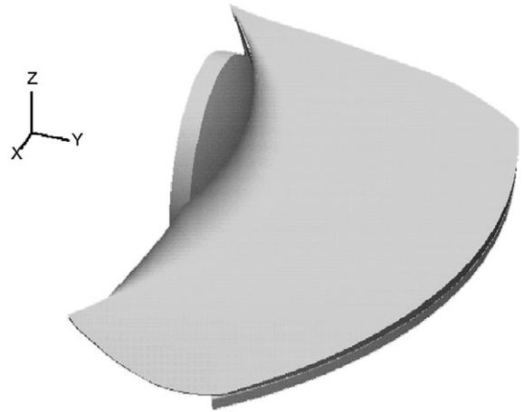
Fig. 2. 3D modeling of Kaplan turbine blade.
