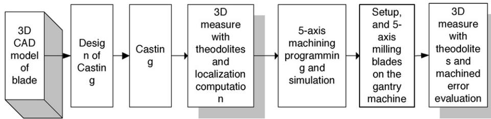
Fig. 1. A typical blade manufacturing strategy for large size hydro turbines.
