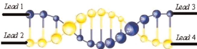
Fig. 1. Four-terminal circuit based on the DH molecule coupling to four normal metallic leads.
