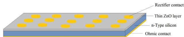
Fig. 1. The schematic of Au/ZnO/n-Si structure.
