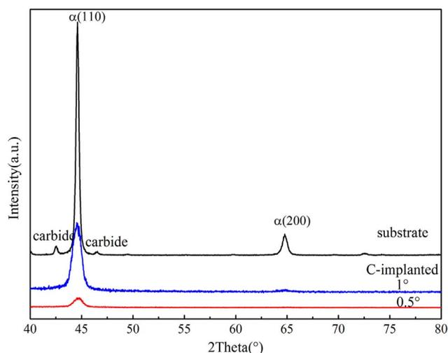
Fig. 2. GAXRD diffractograms in the 40–80° diffraction angles region acquired at  $0.5^\circ$  and  $1^\circ$  for the non-implanted and carbon implanted M50NiL.
