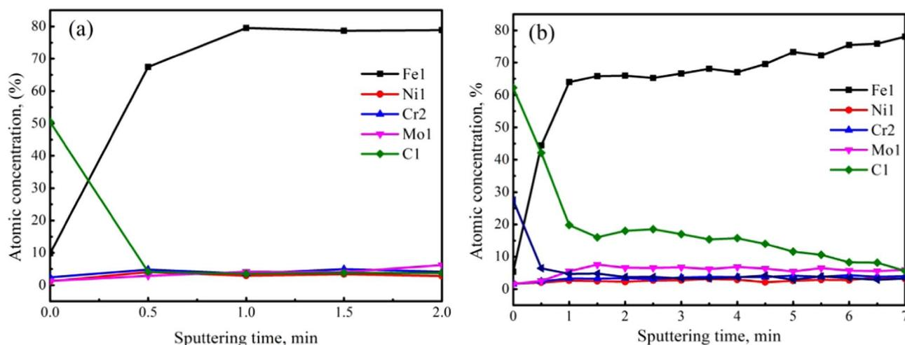
Fig. 1. Depth profile acquired from (a) substrate and (b) carbon implanted M50NiL sample, using AES.
