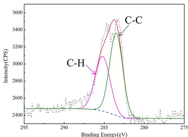
Fig. 3. C1s XPS spectra at the depth of 3 nm for carbon-implanted M50NiL steel.
