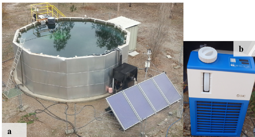
Fig. 1. Solar pond pilot plant in Martorell: (a) the solar thermal collectors used in the heat supply experiments and (b) cooler system used in the heat extraction test.
