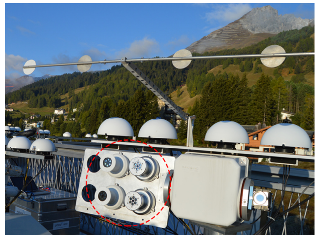
Fig. 1. SolarSIMs, versions D1 and D2, installed on a Brusag tracker on the roof top at the World Radiation Center, Davos, Switzerland (white finish - SolarSIM-D1, silver finish - SolarSIM-D2). (For interpretation of the references to color in this figure legend, the reader is referred to the web version of this article.)
