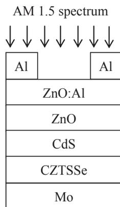
Fig. 1. The basic structure of CZTSSe thin film solar cell used in the calculation.
