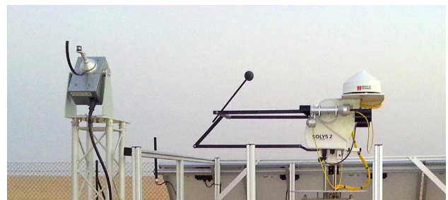
Fig. 1. Detail of the experimental setup, pictured at sunrise, showing an RSI (left) and thermopile radiometers mounted on a sun tracker with shading-ball attachment (right). The backside of PV solar panels (needed to power such an autonomous station) appears in the bottom right part of the picture.
