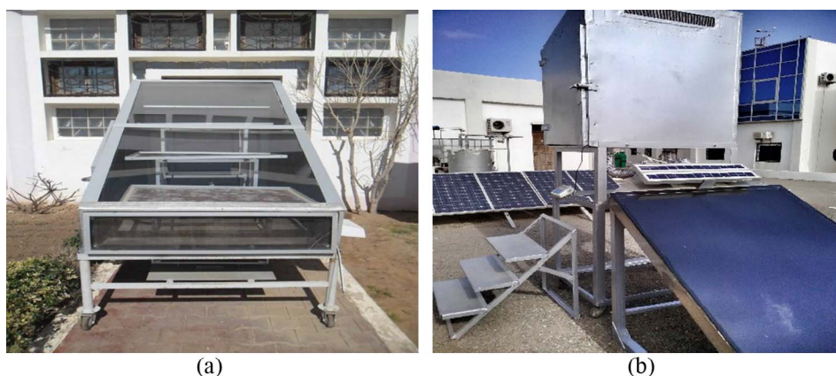
Fig. 1. Solar dryers: (a) DSD; (b) ISD.
