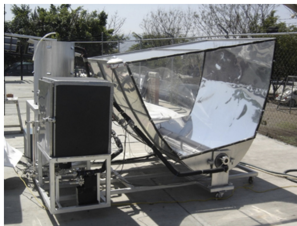
Fig. 1. Photograph of the solar intermittent absorption refrigeration system analyzed.
