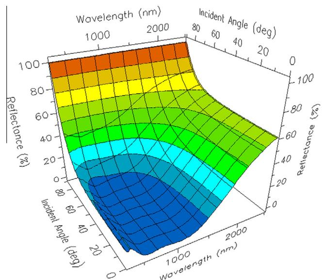
Fig. 1. Simulated reflectance spectra of Mo–SiO<sub>2</sub> double cermet absorber coating at different incident angles from 0° to 90°.
