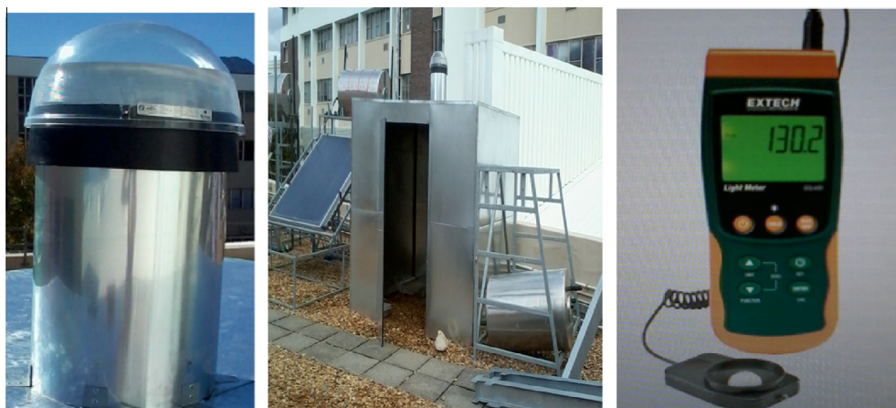
Fig. 1. Experiment equipment; light pipe, sheet metal box and light meter.
